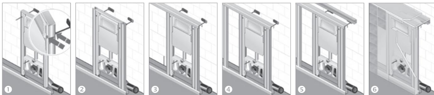
① Fasten the U-profile to the floor at the required distance to the wall and place the BS+ element into it. Install the two wall brackets supplied as accessories to the BS+ element and adjust the gap between the element and the wall with the aid of the wall brackets. Make the wall brackets face downwards or to the side. Cut the threaded rods off so that they no longer protrude from the element. Tighten the lock nuts.
