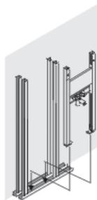
Inserting the element into the stud wall.
