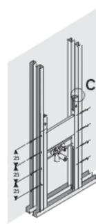
Screw the aligned stud wall panel combination to the side and to the floor.
