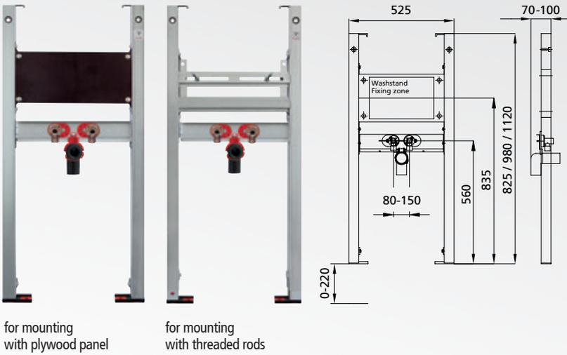
for mounting with plywood panel
