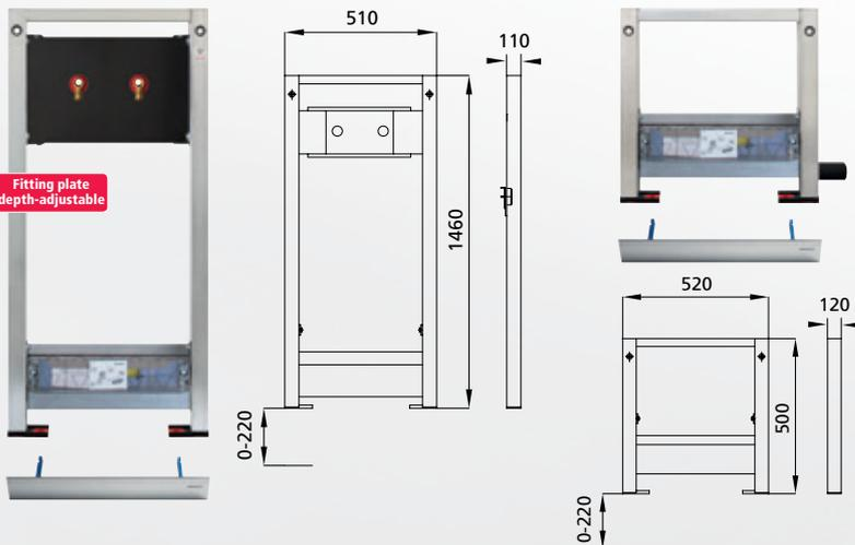
For installation in a stud wall in accordance with DIN 18183 or in conjunction with accessory set art. no. 240012 as a single element in a pre-wall installation.
