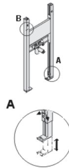
Height adjustment of the element is done by adjusting the feet of the element. (A)
