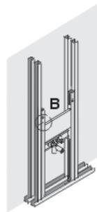
Metre mark on the stud wall align with the marking on the panel. (B)
