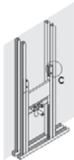
Align the outer edges of the element flush with the outer edges of the stud wall and fix the position. (C)
