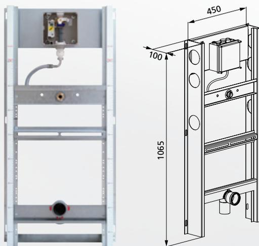
**Complete pre-assembled installation unit for brickwork made of galvanised steel frame.**
