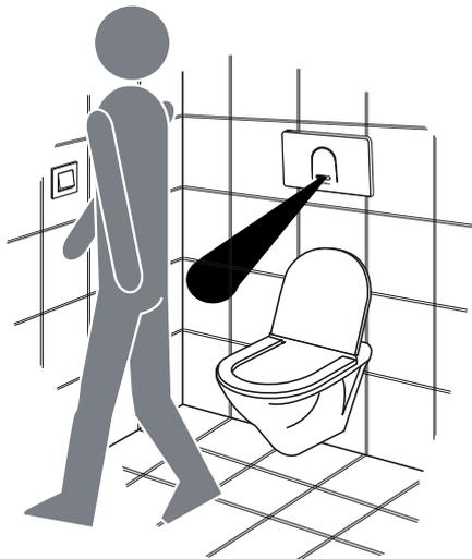
Automatic flushing after leaving the WC (switchable) Minimum stay time 15 s
