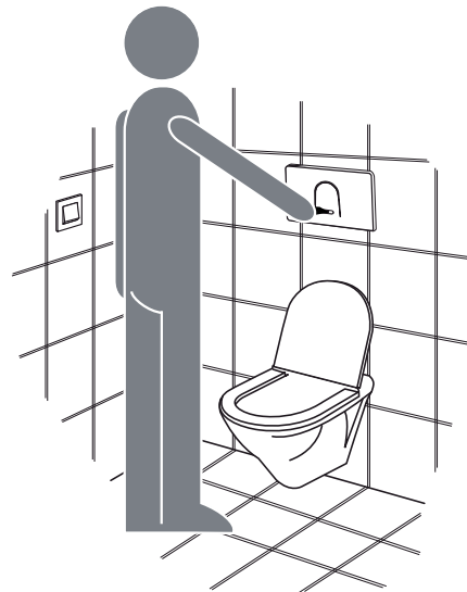
Contactless manual flush can be activated by approaching the hand to the capacitive-infrared sensor
